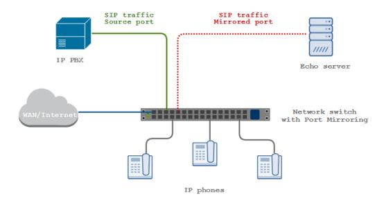
Your telephone system will be connected to one port on your managed switch, sourcing the SIP traffic, which will then be configured to send a copy of all SIP packets to another port, connected to one of the network cards on the Echo server.
