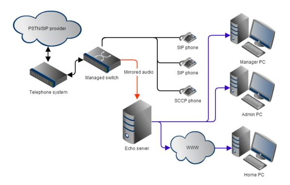
Monitoring handsets that are capable of either SCCP or SIP communication allow generic recording to occur, regardless of what combination of PSTN interfaces are in use, e.g. SIP, PRI, BRI, analogue.
