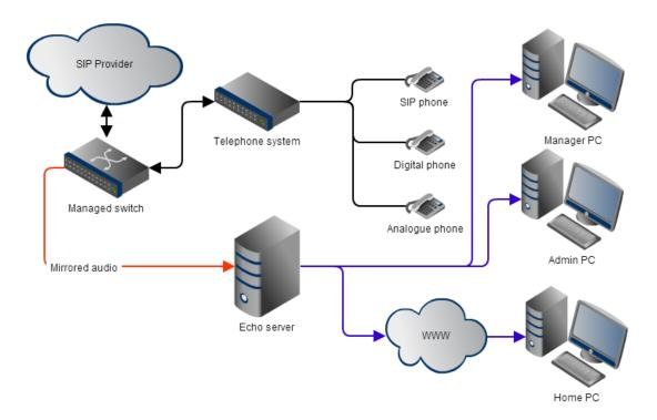
Monitoring SIP trunks allows any phone system or handsets to be recorded. This includes proprietary handsets which would normally be expensive when recording extension-side.
