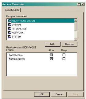
5. Next step is to modify the way DCOM behaves on the computer by executing the DCOM configuration program: Start -> Run ->
